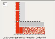
foundation slab with perimeter insulation brick and perimeter insulation
