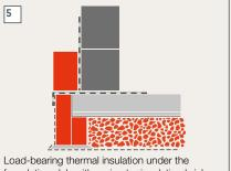
foundation slab with perimeter insulation brick and base insulation
