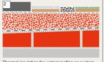
Thermal insulation for waterproofing as system solution with a combination of GLAPOR insulating gradient boards and GLAPOR lightweight gravel
