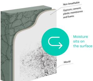
Condensation forms on cold surfaces, leading to mould growth.
