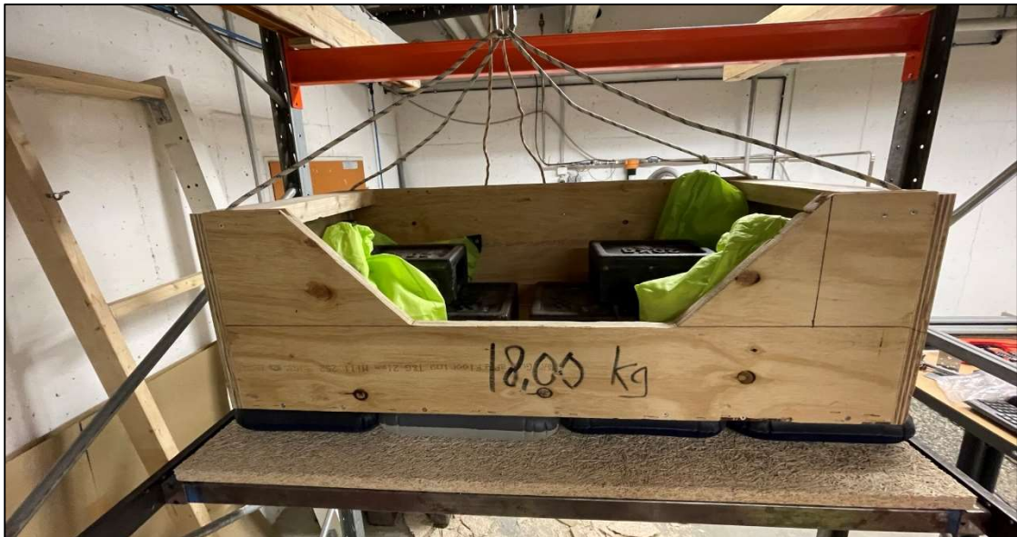
Photo 2. Specimen applied with 80% preload
